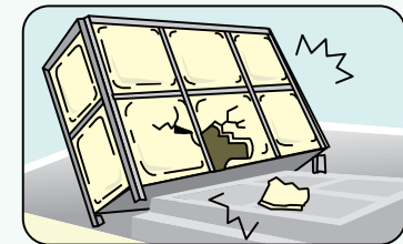
5 Check the outward appearance of the water tank. Is it damaged?
