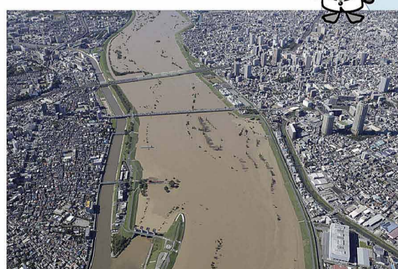
Arakawa River After Typhoon Hagibis (Typhoon 19 of 2019) passed through (Near Kita City, Iwabuchi Floodgate on October 13 around 1PM Approx. A.P.+7.01m (Approx. 70 cm lower than the flood danger water level))
